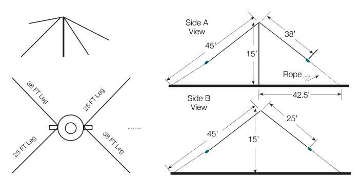
The EZ NVIS is ready to deploy NVIS antenna based on an article by Carl Jelnick, N6VNG (SK). He based his design on the AS-2259/GR a military, dual band NVIS antenna set. The antenna comes with a center support and the four assembled and marked antenna elements. You need to add rope, coax and an appropriate mast. The antenna is constructed from 14ga Soft Drawn copper wire.
