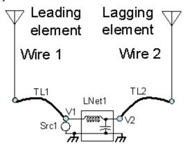
Of course, transmission lines TL1 and TL2 each have two conductors, and the models have two sets of two terminals just like the L network object LNet1. The second conductor is omitted from the diagram for simplicity.
