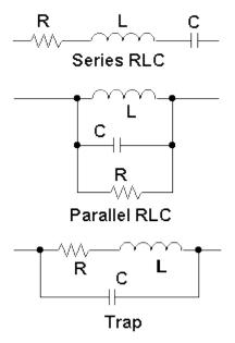
Values of R, L, and C are entered in the appropriate columns. **EZNEC** will calculate and use the impedance of the RLC combination as required.
