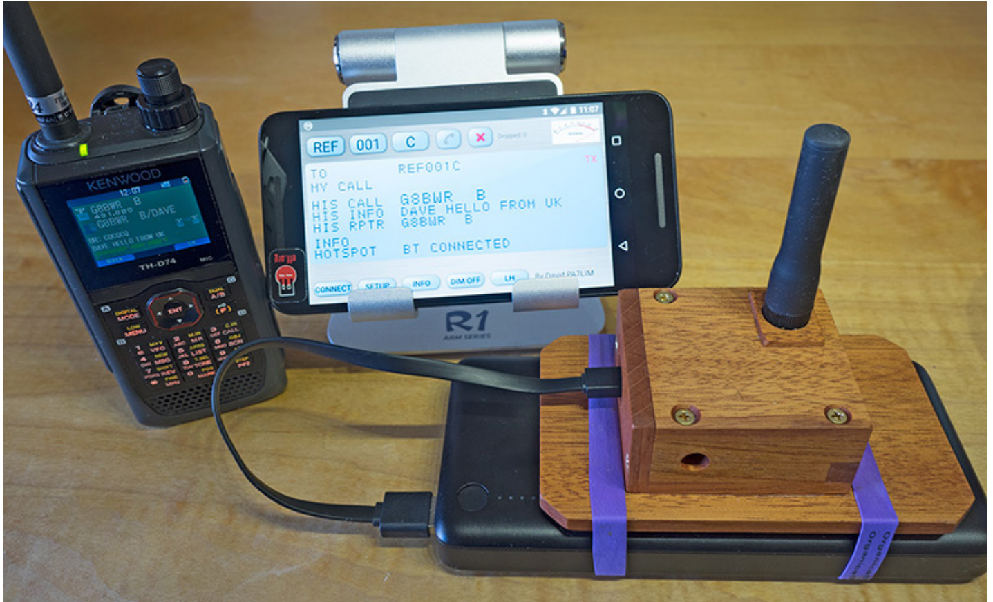
I made a case for the BlueStack-DVMEGA duo out of some mahogany scraps
