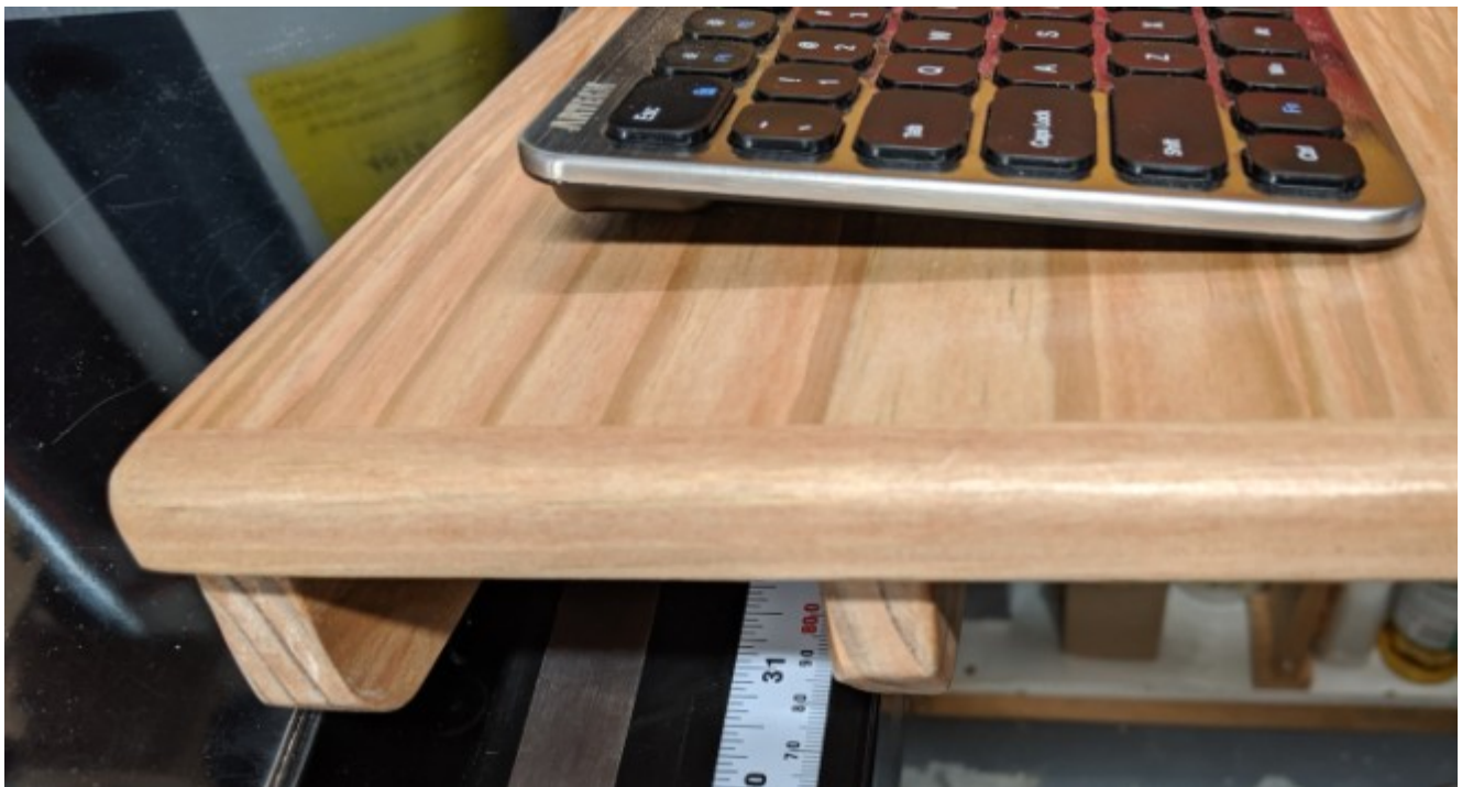
Side view of the keyboard tray (partially lifted up) showing how it mounts:
